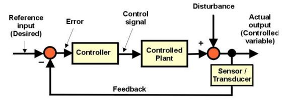
Fig.15: Feedback control system
