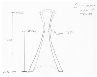
of R<sub>in</sub> is 3 ft and you set Put-THROUGH the x-coordinate where that occurs (say, 70% of the way up the trunk), then you have one of the needed pairs of x and R<sub>in</sub> for determining a, b, and c. Then, vou select if reasonable values of Rin at the top and bottom, you have the two remaining pairs of x and R<sub>in</sub> that you need to solve for a, b, and c. Do a similar thing for three pairs of x and R<sub>out</sub> values and you can solve for d, e, and f.
