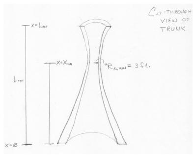
of  $R_{in}$  is 3 ft and you set Put-THROUGH the x-coordinate where that occurs (say, 70% of the way up the trunk), then you have one of the needed pairs of x and R<sub>in</sub> for determining a. b. and c. Then, vou select if reasonable values of Rin at the top and bottom, you have the two remaining pairs of x and R<sub>in</sub> that you need to solve for a, b, and c. Do a similar thing for three pairs of x and R<sub>out</sub> values and you can solve for d, e, and f.
